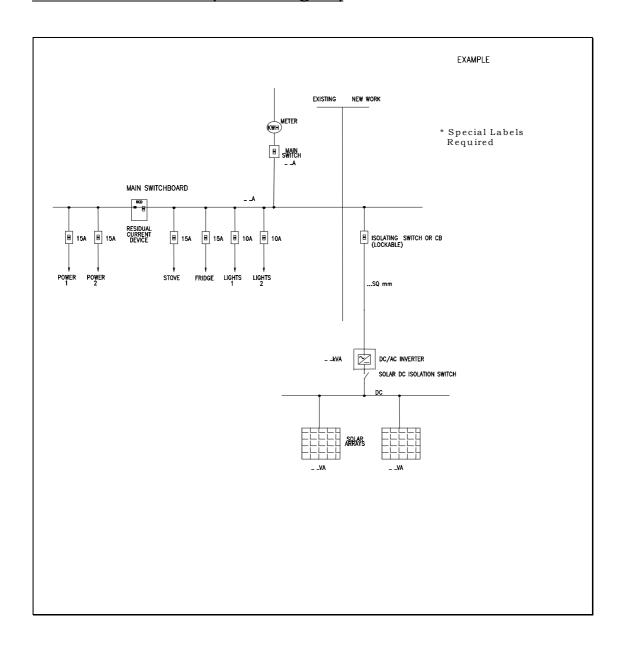
Typical label to be installed at Main Switchboard or Distribution Board where the inverter energy system is connected
