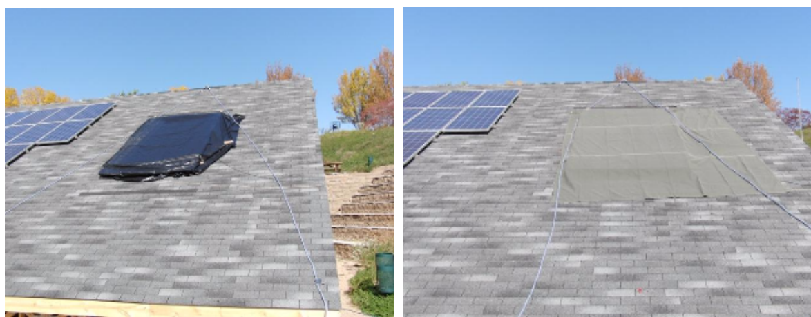
Figure 16: Underwriters Laboratories Tarp Experiment (Backstrom & Dini, 2011)
