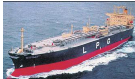
Figure 11: LPG carrier suitable for ammonia. Source: http://www.liquefiedgascarrier.com
