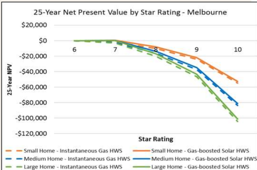
Figure 37: 25-Year NPV by Star Rating/Size, Dual Fuel Home, Melbourne, no Solar PV (7% Discount, High Build Cost Premium)
