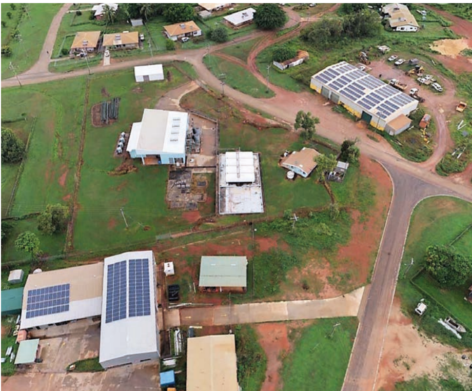
The 209kW Lockhart River Solar Battery Trial on the Cape York Peninsula includes a 60kWh battery backup system and was financed with a renewable energy loan from Indigenous Business Australia.
